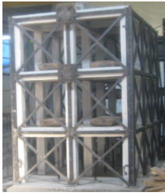
Figure 7. Retrofitted by exterior steel brace system model
